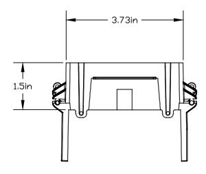
ETL Listed Conforms to UL Std. 514C Single gang low voltage bracket Designed to fit a standard single gang faceplate Mounts with nails All dimensions are nominal
