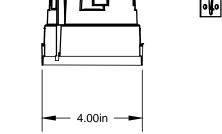
ETL Listed Conforms to UL Std. 514C 2-HR Fire Ceiling Rating ETL Control # 3107144 Material is Polycarbonate 25 Cubic Inches Volume Ceiling Fixture Box with Ground Lug 50Lb. Maximum Fixture Weight Not for ceiling fan installation Mounts with hanging bar
