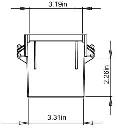
ETL Listed Conforms to UL Std. 514C 2-HR Fire Wall Rating ETL Control # 3107144 Mounts with nails Material is Rigid PVC All dimensions are nominal
