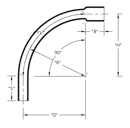
**CONFORMS TO NEMA TC 6&8** MATERIAL IS HIGH MODULUS (HM) 500,000 psi BEND TOLERANCE IS ±2° "B"TOLERANCE IS - 1/8", + 1/2"
