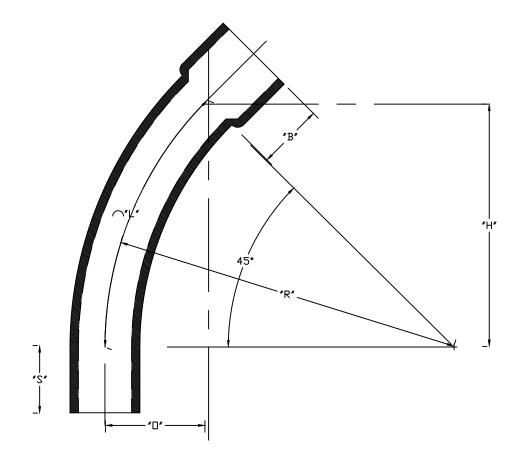
NOT A LISTED PRODUCT CONFORMS TO NEMA TC 3 MATERIAL IS RIGID PVC BEND TOLERANCE IS ±2°
