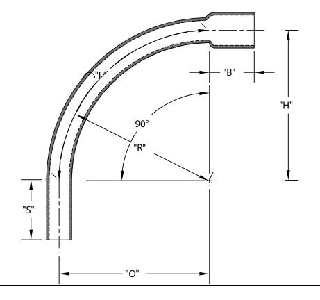
**ETL LISTED CONFORMS TO UL651** ETL CONTROL #3107144 **CONFORMS TO NEMA TC3** SEE NEC ARTICLE 352 FOR USE MATERIAL IS RIGID PVC BEND TOLERANCE IS ±2° "B" TOLERANCE IS -1/8", +1/2"
