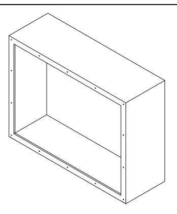
Not a UL Listed Product UL-94 V-O Flame Rating Material is Rigid PVC NEMA 4X Rating Meets or exceeds NEMA 250 Stds. Cover is fully gasketed
