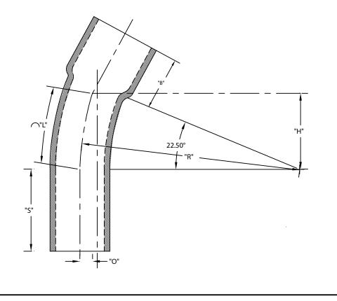
CONFORMS TO NEMA TC 6&8 MATERIAL IS HIGH MODULUS (HM) 500,000 psi BEND TOLERANCE IS  $\pm 2^{\circ}$ "B"TOLERANCE IS  $- \frac{1}{2}$ "
