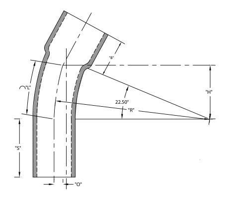
CONFORMS TO NEMA TC 6&8 MATERIAL IS HIGH MODULUS (HM) 500,000 psi BEND TOLERANCE IS  $\pm 2^{\circ}$  "B"TOLERANCE IS -1/8", +1/2"
