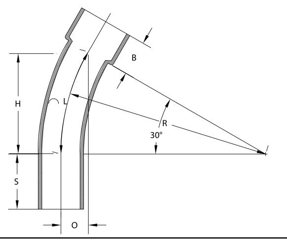
CONFORMS TO NEMA TC 6&8 MATERIAL IS HIGH MODULUS (HM) 500,000 psi BEND TOLERANCE IS  $\pm 2^{\circ}$  "B" TOLERANCE IS  $-\frac{1}{8}$ ",  $+\frac{1}{2}$ "
