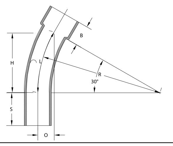
CONFORMS TO NEMA TC 6&8 MATERIAL IS HIGH MODULUS (HM) 500,000 psi BEND TOLERANCE IS  $\pm 2^{\circ}$  "B"TOLERANCE IS  $-\frac{1}{2}$ ",  $+\frac{1}{2}$ "
