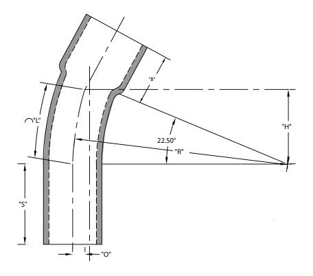
**CONFORMS TO NEMA TC 6&8** MATERIAL IS HIGH MODULUS (HM) 500,000 psi BEND TOLERANCE IS ±2° "B"TOLERANCE IS -1/8", +1/2"
