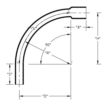
NOT A LISTED PRODUCT CONFORMS TO NEMA TC 3 MATERIAL IS RIGID PVC BEND TOLERANCE IS ±2°
