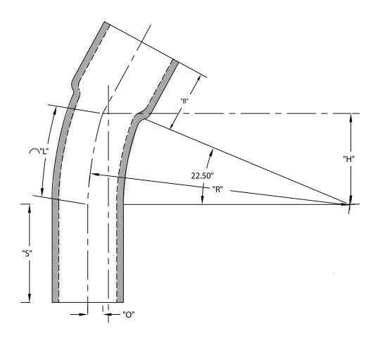
CONFORMS TO NEMA TC 6&8 MATERIAL IS HIGH MODULUS (HM) 500,000 psi BEND TOLERANCE IS  $\pm 2^{\circ}$  "B"TOLERANCE IS  $-\frac{1}{8}$ ",  $+\frac{1}{2}$ "
