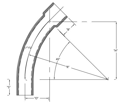
**CONFORMS TO NEMA TC 6&8** MATERIAL IS HIGH MODULUS (HM) 500,000 psi BEND TOLERANCE IS ±2° "B"TOLERANCE IS - 1/8", + 1/2"
