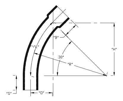
NOT A LISTED PRODUCT CONFORMS TO NEMA TC 6&8 MATERIAL IS RIGID PVC BEND TOLERANCE IS ±2°
