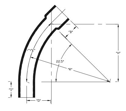
NOT A LISTED PRODUCT CONFORMS TO NEMA TC 6&8 and ASTM F-512 MATERIAL IS RIGID PVC BEND TOLERANCE IS ±2° ALL DIMENSIONS ARE NOMINAL
