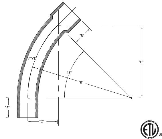
ETL LISTED CONFORMS TO UL651 ETL CONTROL #3107144 CONFORMS TO NEMA TC3 SEE NEC ARTICLE 352 FOR USE MATERIAL IS RIGID PVC BEND TOLERANCE IS ±2° "B" TOLERANCE IS -½", +½"
