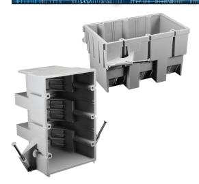
EZ53TN-HW is a 3-gang, 53 cu. in., heavy wall EZ BOX that is ideal for new work applications for residential and light commercial projects where an even more durable box is preferred. The harder shell is designed to resist flexing and hold its shape. It features enhanced, angled nails for easy mounting between studs and 12 integral wire clamps for EZ secure wiring.
