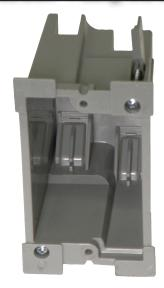
EZ18SO-HW is a 18 cu. in., 1-gang, old work, heavy wall electrical switch and outlet EZ BOX for renovation projects (old work). This heavy duty box with EZ mount flanges and winged mounting tabs is perfect for residential and light commercial applications where a more durable shell is desired. The harder shell resists flexing in various conditions. Wing tabs allow for easy, secure stud alignment & mounting.
