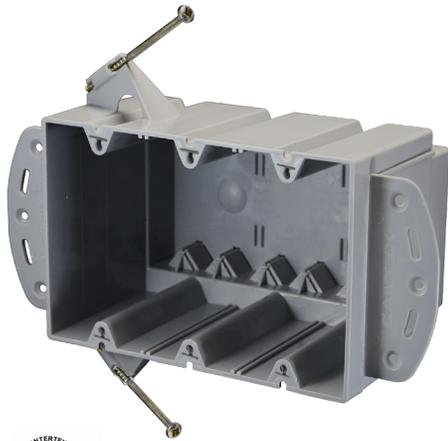
EZ74TNZU EZ BOX is a 74 cu. in., deep, 3-gang switch and outlet box for residential or light commercial new construction (new work) installations. It features molded brackets for steel stud mounting along with v-clamps, Express Clips® and screw-nails for EZ installation. The sharp point, slotted head and threaded body of screw-nails allow for installation with a power screwdriver without having to pre-drill aluminum, light to medium grade steel or wood studs.
