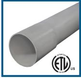
"D" "" **Part** Feet per "B" "E" "OD" Size Pack No. Min Min. Min. A77CA42 .060 1.750 2 2,800 2.375 2.396 2.378 240 A77DA42 3 1,760 .061 3.500 3.529 3.503 2.875 240 A77EA42 4 1,140 .082 4.500 4.533 4.502 3.375 240 A77FA42 5 760 .103 5.563 5.601 5.562 4.000 240
